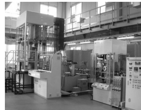
SPS Job-shop center in Japan (left/3MN right/200KN) φ300mm large Al 2 O 3 SPSed compact(Relative density:98%)
